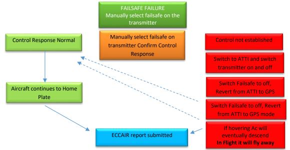
e. **Fly Away Actions**. Should the aircraft fly beyond the range of the transmitter the GCS / MC will automatically apply the Failsafe mode. In this mode, the aircraft will operate as previously discussed. If the aircraft continues to fly away the PiC is to carry out the following actions:
